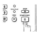
■ When copy completes, the fax machine sounds several beeps. To copy more documents, insert the next sheet while the fax machine is beeping. The fax machine makes a copy of the next sheet.
